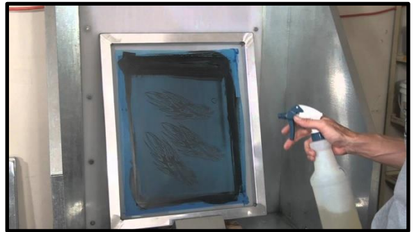
FRAME CLEANING WITH REDUCER
